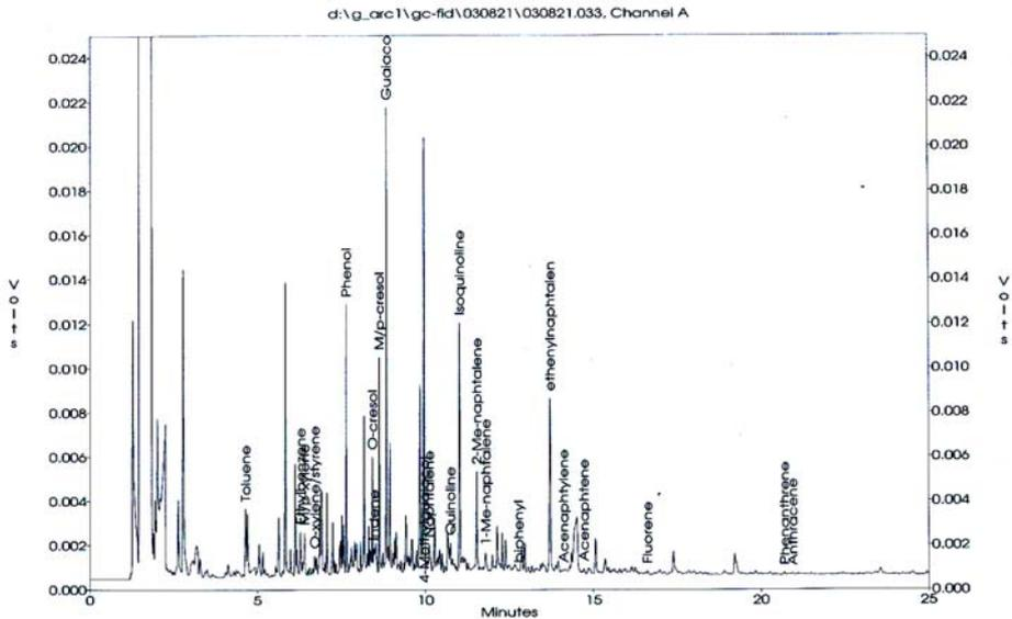
Figure 2- GC Chromatograms of updraft gasifier tar sample. The Technique used is GC-FID, apolar column. It is recognisable that peak separation is not clear, and no clear baseline visible in the most of the chromatogram [9].
