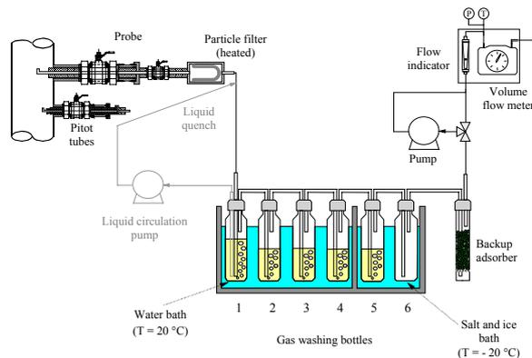
Figure 1: The Guideline sampling set-up: atmospheric and isokinetic sampling train for tar and particles with removable probe and pitot tubes for flow measurement.
