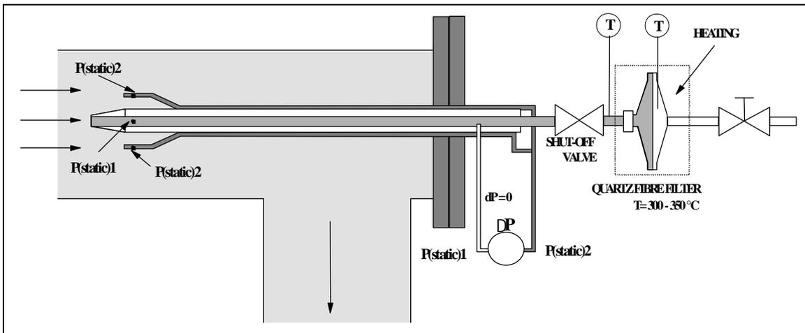
Figure 6-2 The configuration of the O-type probe
