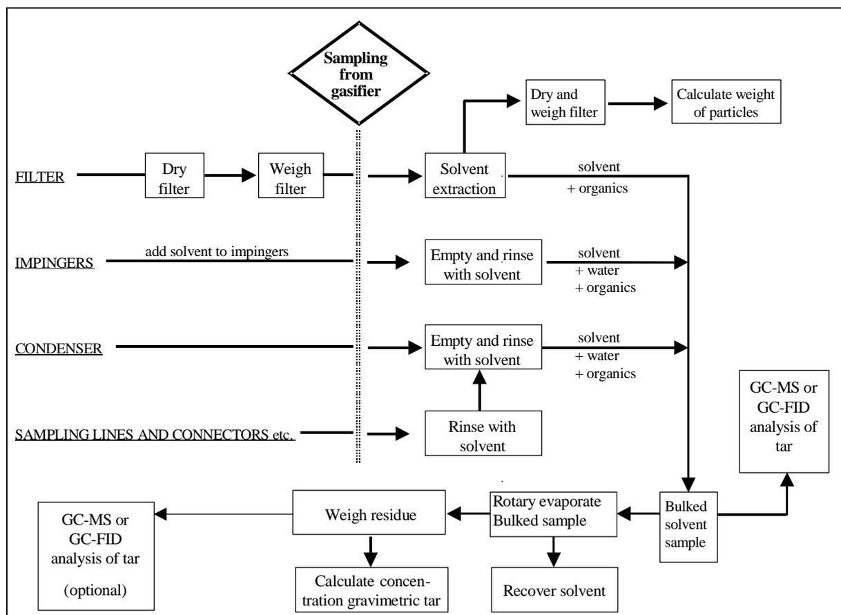
Figure 8.1 Schematic Showing Post Sampling Procedures
