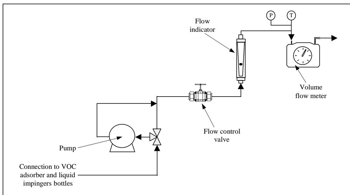
Figure 5-6: Pump and flow measuring equipment in Module 4.
