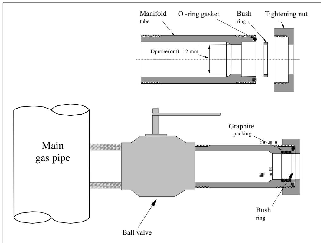
Figure 6-3: Sampling port with lock consisting of ball valve and stuffing box (the sampling probe is not shown)
