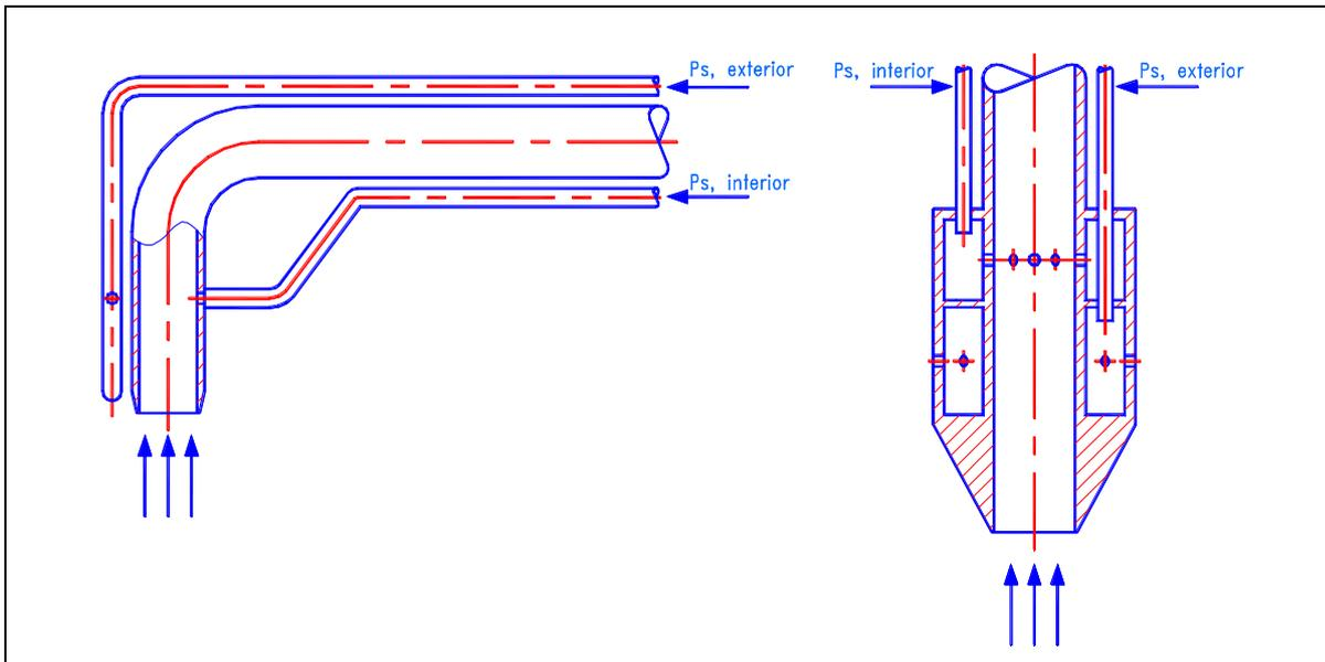
Figure 7-1 Simple O-type probe
