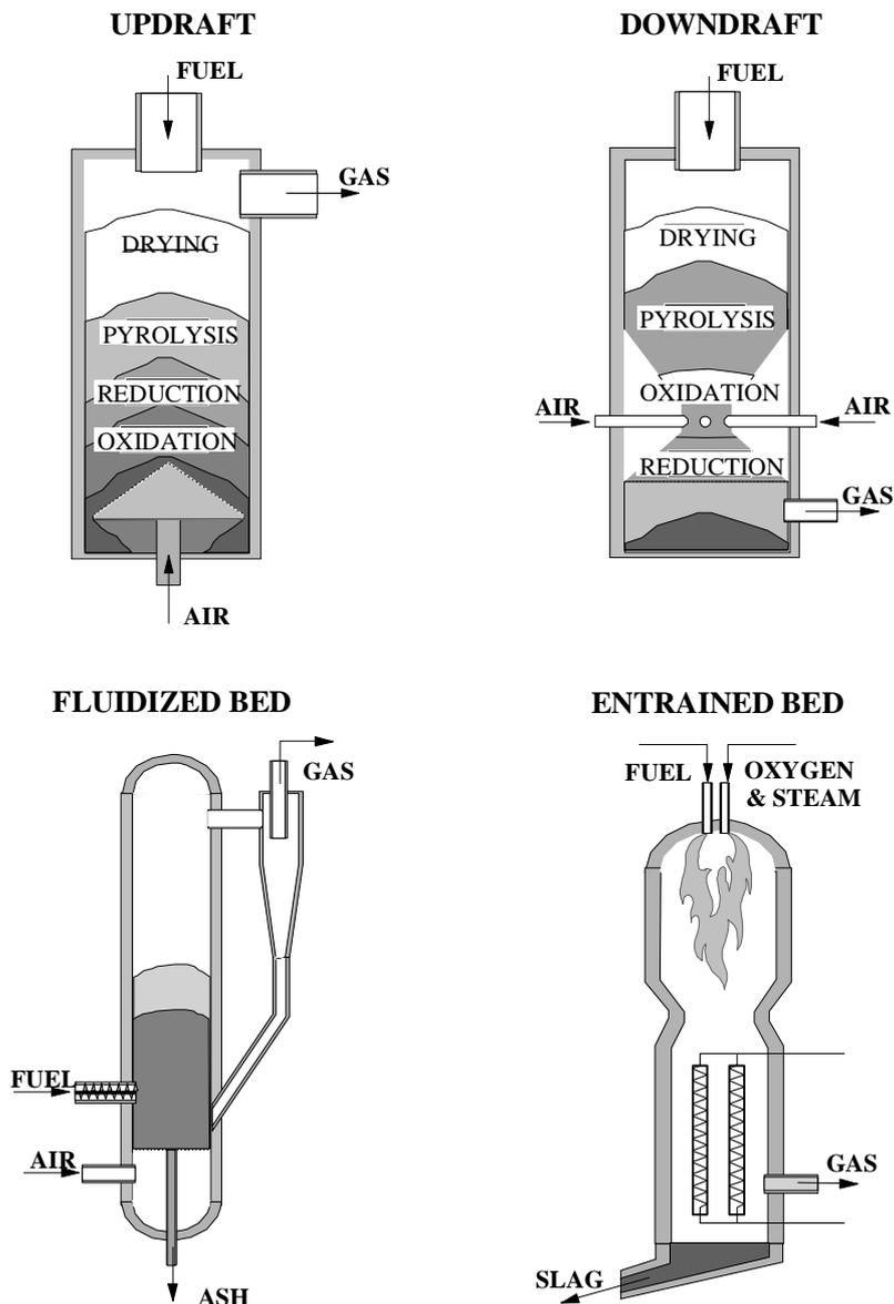
Figure 13-1: Schematic drawing of four basic gasifier types
